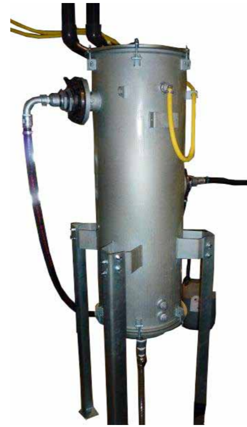
Vapor Extraction in Vacuum Extrusion
